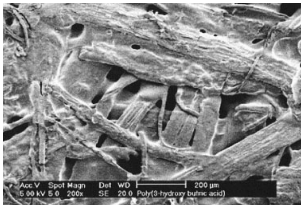
Figure 2 SEM image of PHB-flax composite surface morphology; good surface wetting is characteristic for these biopolyesters.
